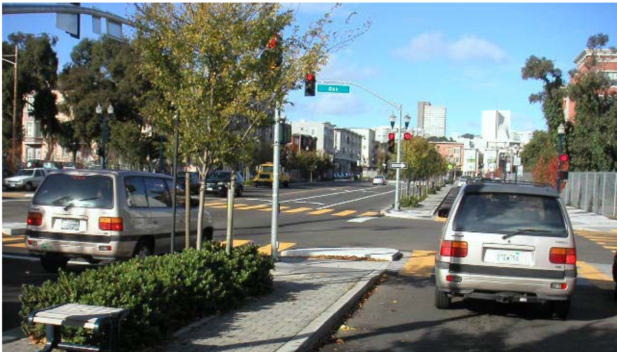
OCTAVIA AT OAK: CAR ON THE RIGHT CAN PROCEED STRAIGHT WHILE THE CAR ON LEFT MAKES A RIGHT TURN
