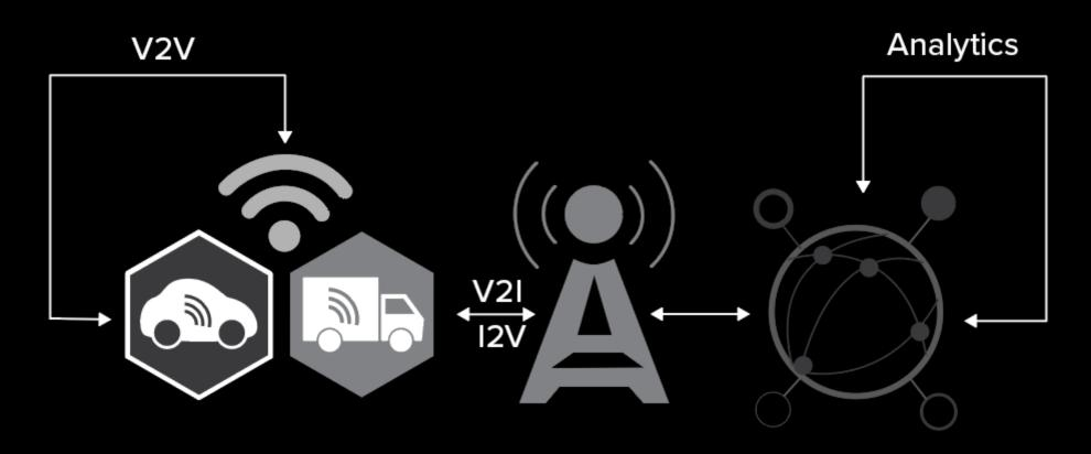
On-board Equipment (OBE) Subsystem Roadside Equipment (RSE) Subsystem V2X Data Ecosystem (VDE) Subsystem
